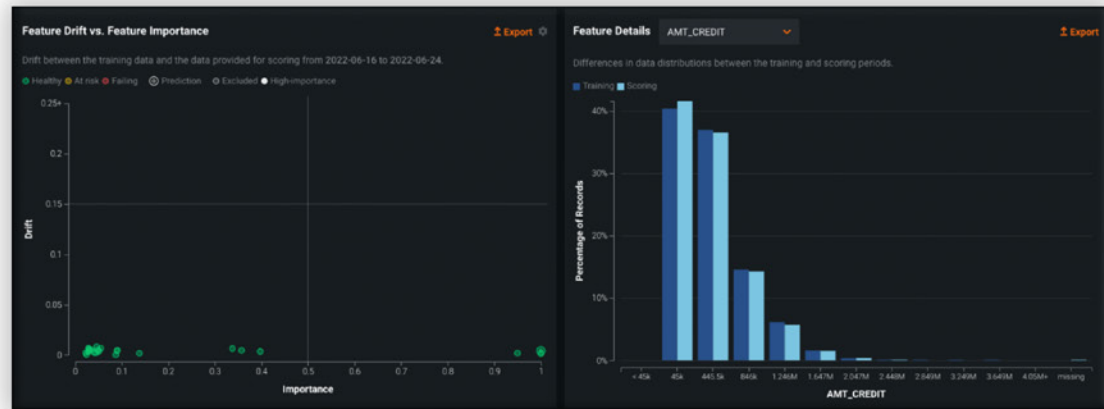
Figure 13: Data drift tab of a deployed DataRobot model. Left-hand image depicts a scatter plot of Feature Drift vs. Feature Importance. The right-hand image depicts a histogram of the frequency of values observed in a live setting vs. when the model was trained.
