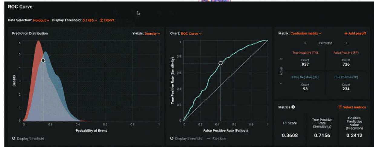
Figure 10: DataRobot provides an interactive ROC curve specifying relevant model performance metrics on the bottom right.
